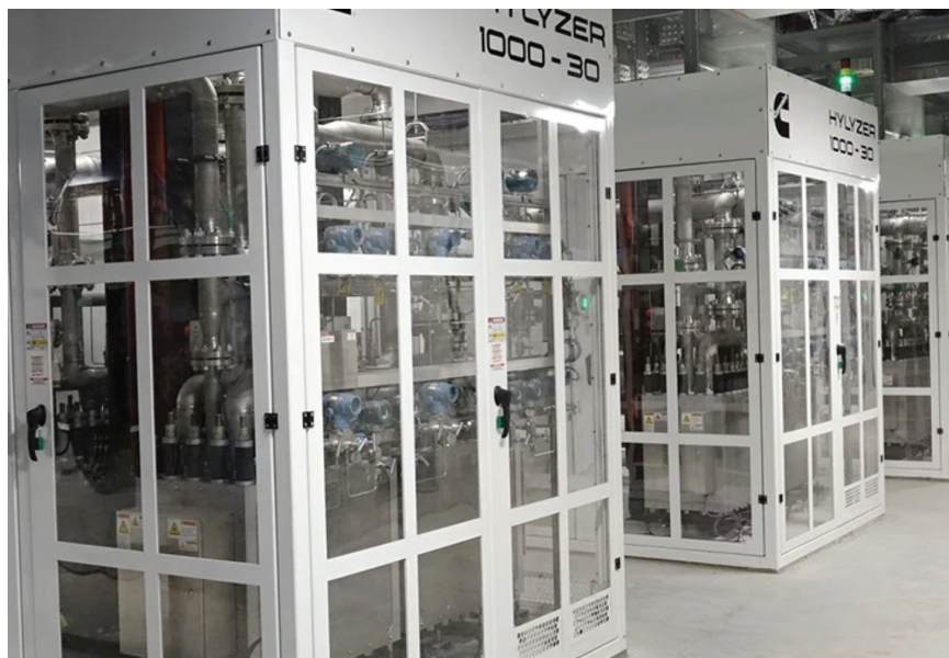
FIGURE 3.4 HyLYZER® proton exchange membrane electrolyzer system installed at the Air Liquide hydrogen production facility in Bécancour, Quebec, and producing 3,000 tons of hydrogen annually using clean hydropower. SOURCE: Cummins, Inc., 2021, “Cummins Hydrogen Technology Powers the Largest Proton Exchange Membrane (PEM) Electrolyzer in Operation in the World,” January 26, https://www.cummins.com/news/releases/2021/01/26/cummins-hydrogen-technology-powers-largest-proton-exchange-membrane-pem .
