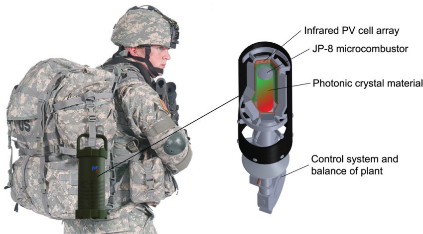
FIGURE 5.4 Notional SSP Concept for soldier-wearable power and cutaway concept. SOURCE: W. Chan, I. Celanovic, and J. Joannopoulos, 2020, “Silent Lightweight Battlefield Power Source: Scalable from Soldier Wearable Power to Platform Power,” white paper presented to committee, Massachusetts Institute of Technology Institute for Soldier Nanotechnologies.
